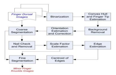
Fig. 5 Block Diagram of proposed work
