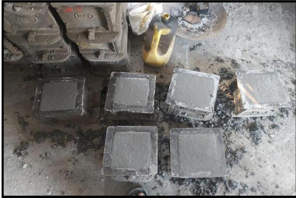
Fig No. 4.1 Casting of cube
