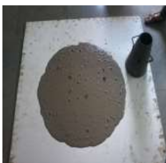
Fig. 2 workability Test on Self Compacting Concrete
